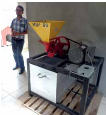
The pulping machine removes the coffee husk, isolating the beans for more efficient processing and improved quality.
